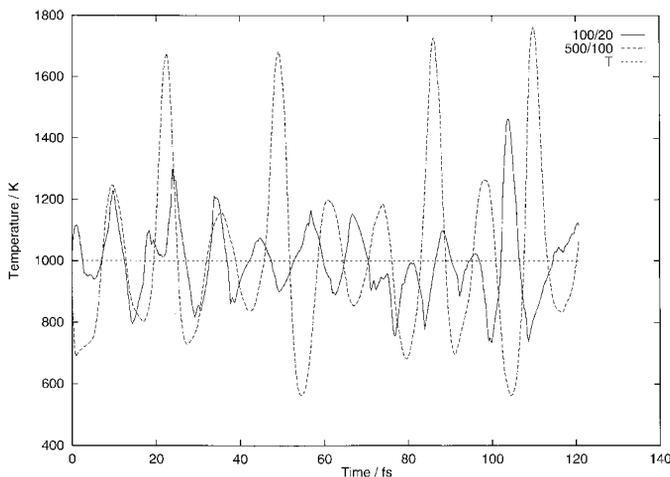
Figure 5. Instantaneous temperature along the trajectories from figure 4. The relative jaggedness of the curve for the trajectory with lighter bath particles probably indicates that the integration is not very good.
