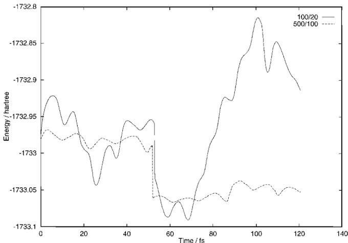
Figure 4. Conserved quantity for two  $\text{Si}_6$  simulations with a time step of 10 au and Nosé–Hoover convergence criterion of  $10^{-20}$ ; one uses masses of 500 and 100 for the bath particles while the other uses masses of 100 and 20. Conservation is significantly better for the trajectory with the heavier bath particles. As before, the discontinuity is due to a sudden change in the electronic state.
