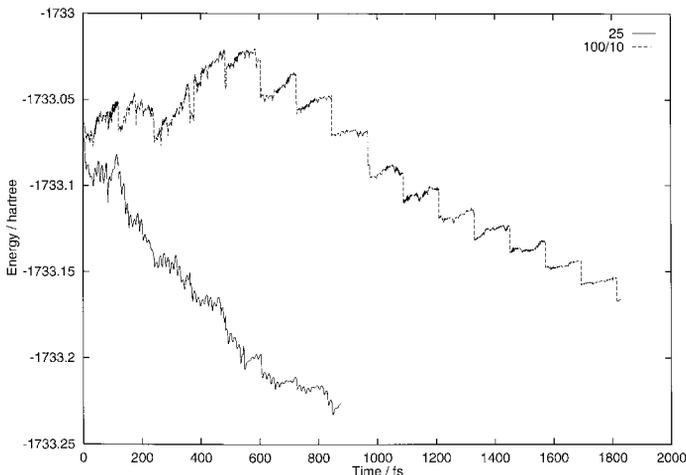
Figure 10. Conserved energy quantity for two annealing trajectories, one with a single time step of 25 atu and one with a time step of 10 atu for the bath particle and 100 atu for the nuclei. Discontinuous drops in energy here are due to periodic temperature reductions.
