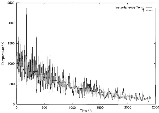
Figure 7. Instantaneous ‘temperature’ of an  $\text{Si}_6$  constant-temperature-based annealing trajectory. The dotted line is the target temperature which appears in the equations of motion.
