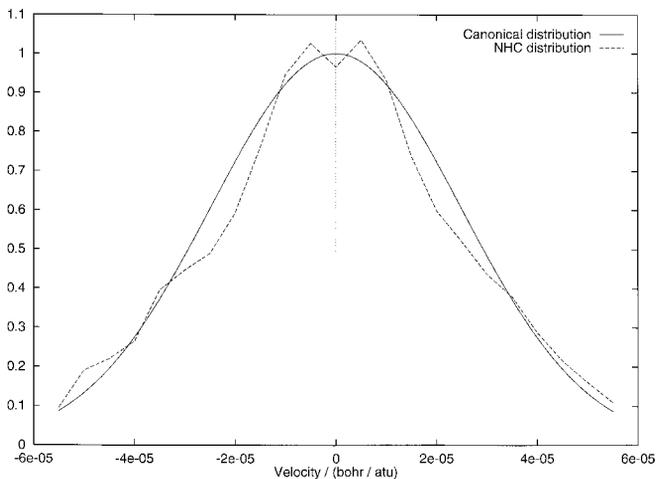
Figure 3. Velocity distribution for a 10 K trajectory with both particle masses of 500 and 100. The solid line is the exact canonical distribution, and the dashed line is the velocity distribution observed in the simulation.
