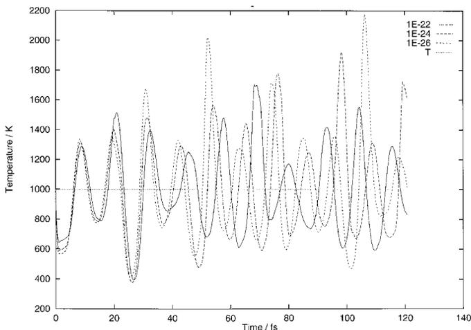
Figure 2. Instantaneous temperature (kinetic energy in units of degrees Kelvin) for the three trajectories with the smallest convergence criteria from figure 1. The line labelled 'T' is the  $T$  which appears in the equations of motion.
