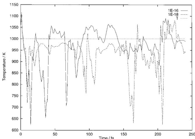
Figure 6. Instantaneous temperature for two trajectories with a time step of 50 atu, and bath particle masses of 100 for the first and 20 for each of the other three; the integration convergence criterion is given in the key. Note the excessive jaggedness of these curves, which shows that the numerical integration is quite poor, as well as the poor distribution of energies (which should be centred around the dotted line labelled ‘T’ at 1000 K).
