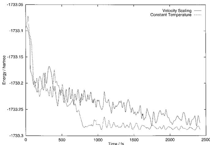
Figure 9. Potential energy of the trajectories from figure 8. Discontinuities observed are due to sudden changes in the electronic wavefunction.
