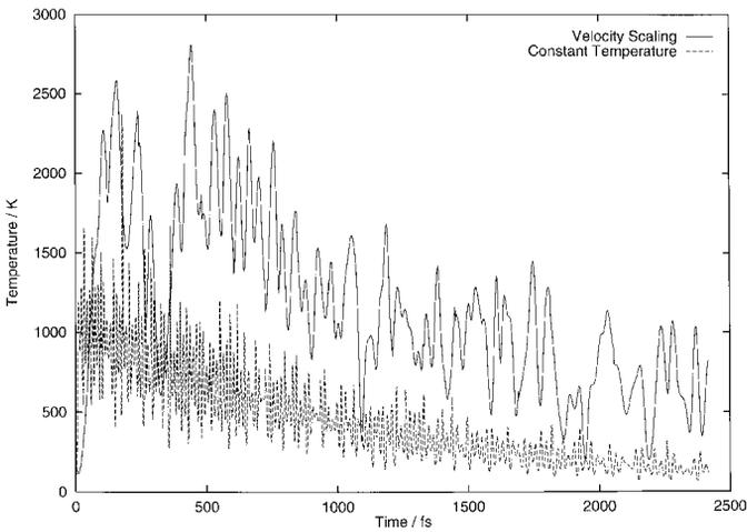
Figure 8. Instantaneous ‘temperatures’ of two  $\text{Si}_6$  annealing trajectories, one with temperature-based annealing and one with velocity-based annealing.
