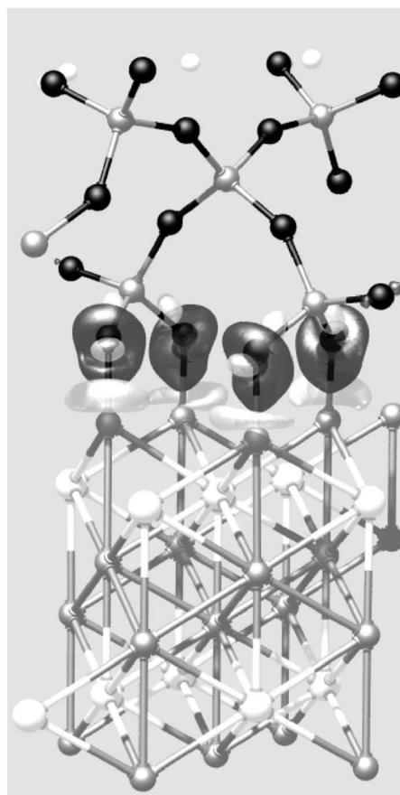
FIG. 6. Isosurface plot of the electron density difference,  $\Delta\rho$ , for  $\text{SiO}_2(100)/\text{MoSi}_2(001)$  interface. The iso-value is at  $-0.075 \text{ e/\AA}^3$  for the light grey surface and at  $0.075 \text{ e/\AA}^3$  for the dark grey surface. Negative  $\Delta\rho$  indicates loss of electron density upon adhesion. Large white balls are Mo atoms, small white balls are H. Si atoms are in grey, and O in black.
