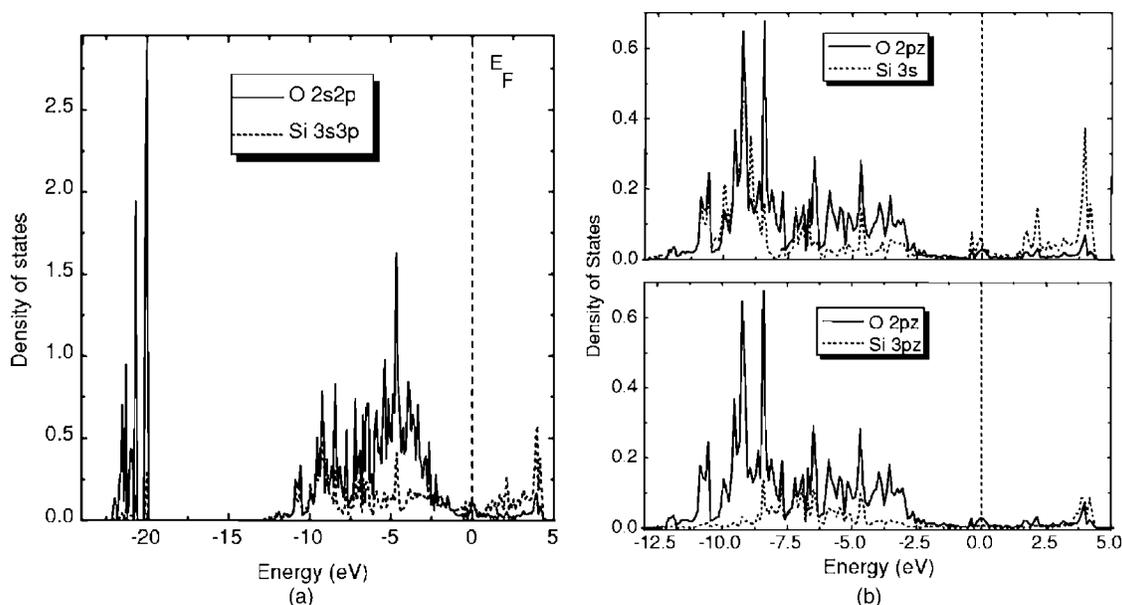
FIG. 5. Site-projected, orbital-resolved local densities of states for Si and O atoms at the  $\text{SiO}_2(100)/\text{MoSi}_2(001)$  interface from Fig. 4(b). The Si atom belongs to  $\text{MoSi}_2(001)$ , while O belongs to  $\text{SiO}_2(100)$ .
