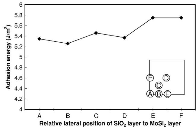
FIG. 3. DFT-LDA adhesion energy vs relative lateral position of the  $\text{SiO}_2(100)$  film to the  $\text{MoSi}_2(001)$  substrate, for a three O-Si-O layer thick  $\text{SiO}_2$  coating. The inset depicts the lateral cell of the  $\text{MoSi}_2$  substrate as a square and the positions of the six different translations of the  $\text{SiO}_2$  coating, with matching points A-F where A is at (0, 0) and D is at (0.5, 0.5).
