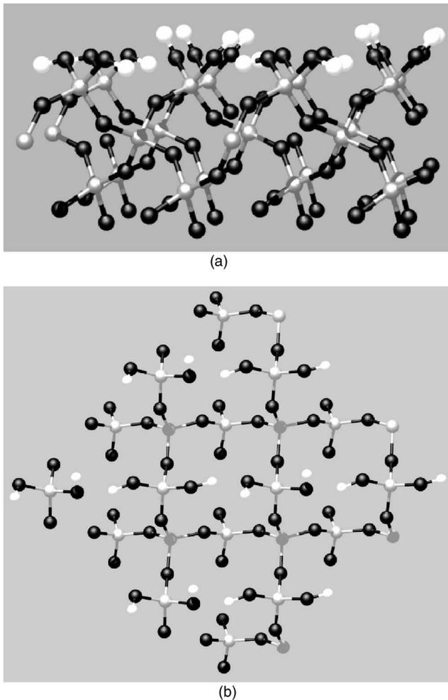
FIG. 2. Side view (a) and top view (b) of the  $\beta$ -cristobalite (100) surface. H atoms are in white, Si in grey, and O in black. The bottom of the surface with unsaturated O atoms is used to adhere to the  $\text{MoSi}_2(001)$  substrate.
