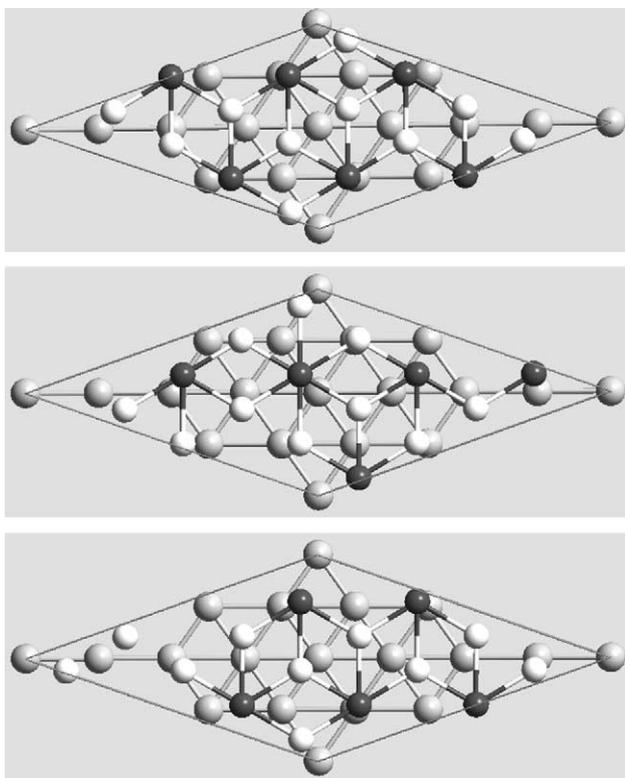
Fig. 7. Three distinct initial structures for relaxation of the  $\text{MoSi}_2(1\ 1\ 0)/\text{Fe}(1\ 1\ 0)$  interface. The resultant ideal adhesion energies are 3.85, 3.78, and  $3.81\ \text{J/m}^2$  for the top, middle, and bottom configurations, respectively.
