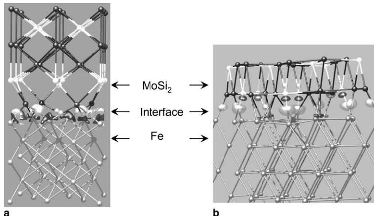
Fig. 5. Isosurface plot of the electron density difference,  $\Delta\rho$ , for (a)  $\text{MoSi}_2(001)/\text{Fe}(100)$  and (b)  $\text{MoSi}_2(110)/\text{Fe}(110)$ . The isosurface values are at  $\pm 0.075 e/\text{\AA}^3$  for (a) and  $\pm 0.10 e/\text{\AA}^3$  for (b). The light grey surface has the positive value, and the dark grey surface has the negative value. Negative  $\Delta\rho$  indicates loss of electron density upon adhesion. Solid balls represent atoms.
