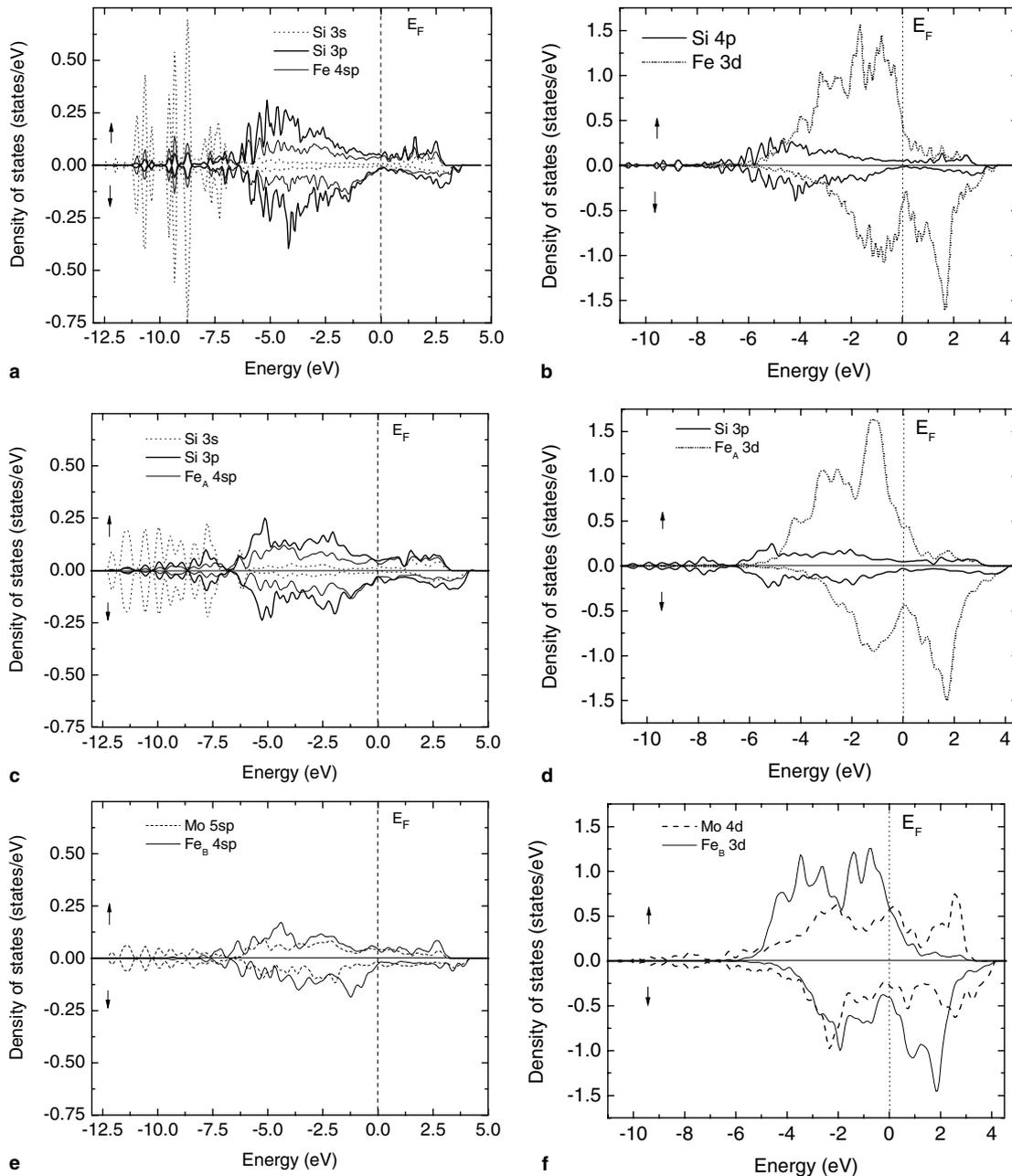
Fig. 6. Spin-polarized local density of states (LDOS) for: a Si atom and a nearest neighbor Fe atom at the MoSi<sub>2</sub>(0 0 1)/Fe(1 0 0) interface [(a) and (b)]; a Si atom and a nearest neighbor Fe atom (Fe<sub>A</sub>) at the MoSi<sub>2</sub>(1 1 0)/Fe(1 1 0) interface [(c) and (d)]; a Mo atom and a nearest neighbor Fe atom (Fe<sub>B</sub>) at the MoSi<sub>2</sub>(1 1 0)/Fe(1 1 0) interface [(e) and (f)].
