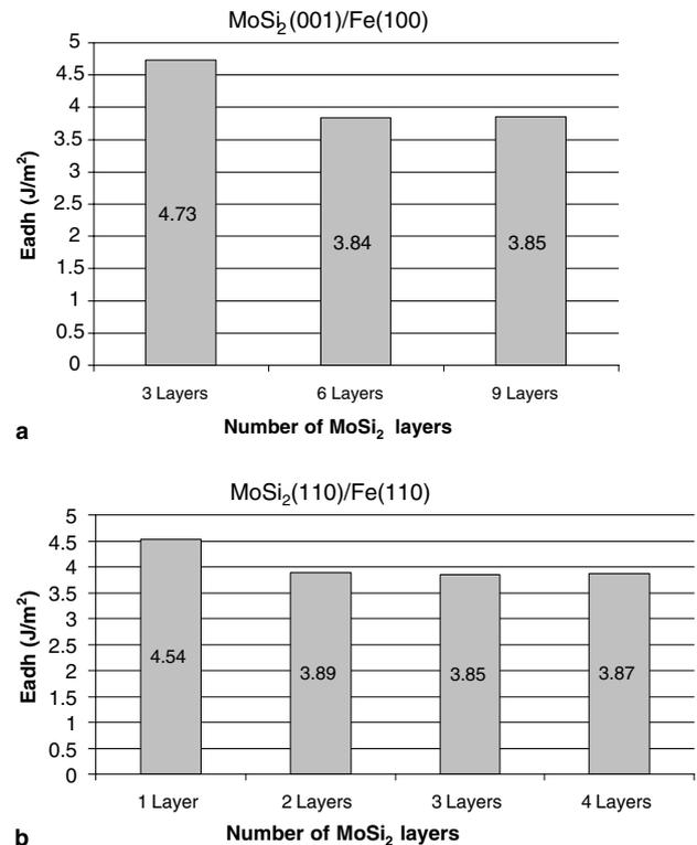
Fig. 3. Convergence of adhesion energy vs. layer thickness: (a)  $\text{MoSi}_2(001)/\text{Fe}(100)$ ; (b)  $\text{MoSi}_2(110)/\text{Fe}(110)$ .
