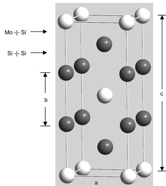
Fig. 1. Bulk structure of MoSi<sub>2</sub>. Si atoms in dark grey and Mo in white.
