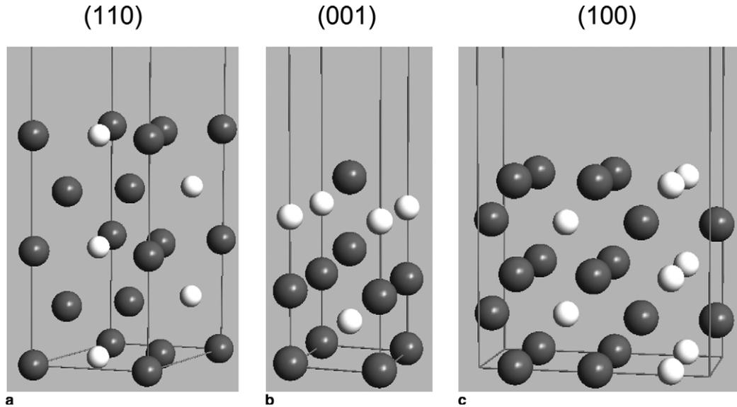
Fig. 2. Surface structures of  $\text{MoSi}_2$ . Si atoms in dark grey and Mo in white.
