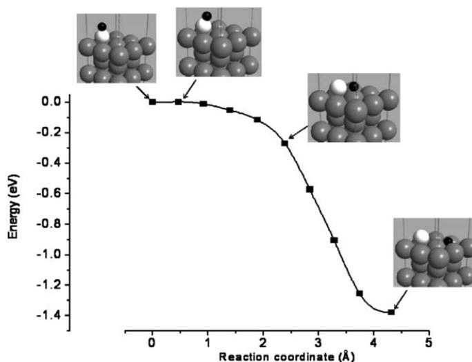
Fig. 6. DFT-GGA minimum energy path for HS dissociation on Fe(110).
