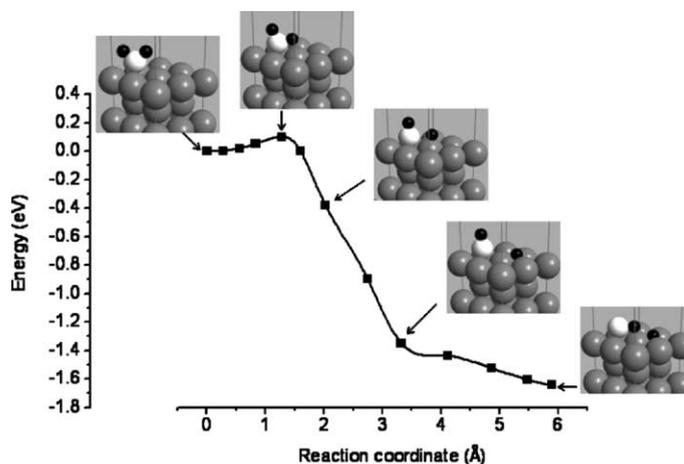
Fig. 5. DFT-GGA minimum energy path for H<sub>2</sub>S dissociation on Fe(110).
