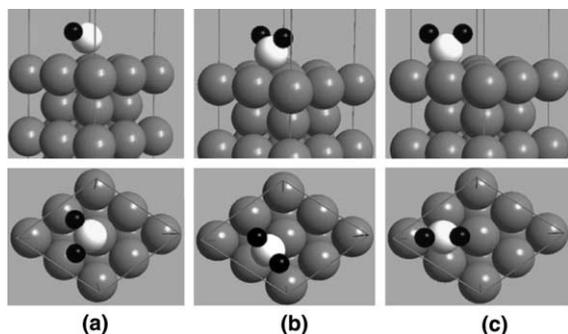
Fig. 2. Lowest energy structures of  $\text{H}_2\text{S}$  adsorbed on high symmetry adsites on  $\text{Fe}(110)$ : (a) on-top; (b) short bridge; (c) long bridge. Upper panel is the side view, and lower panel is the top view. Fe atoms are in grey, S in white, and H in black. The same grey scale convention is used in all subsequent figures.
