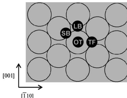
Fig. 1. High symmetry adsorption sites on Fe(110): OT = on-top, SB = short bridge, LB = long bridge and TF = threefold.
