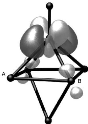
Fig. 4. Isosurface plot of the electron density difference,  $\Delta\rho$ , for HS/Fe(110) in the long-bridge site. Solid black balls represent atoms: the top one is H, the one below H is S, and the atoms below S are Fe atoms. The isosurface value is at  $-0.05$   $\text{e}/\text{Å}^3$  for the light grey surface and at  $0.05$   $\text{e}/\text{Å}^3$  for the dark grey surface. Negative  $\Delta\rho$  indicates loss of electron density upon binding.
