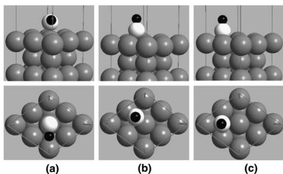
Fig. 3. Lowest energy structures of HS adsorbed on high symmetry adsites on Fe(110): (a) on-top; (b) short bridge; (c) long bridge. Upper panel is the side view, and lower panel is the top view.
