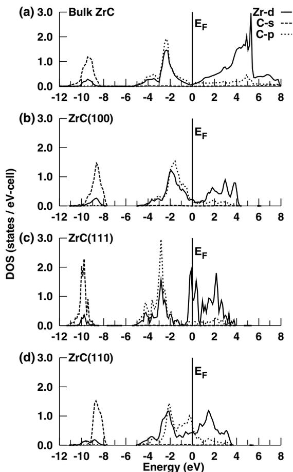
Fig. 2. The *site*- and *l*-projected partial density of states (PDOS) for (a) bulk ZrC, and the surface layer of (b) ZrC(100), (c) metal-terminated ZrC(111) (surface Zr and subsurface C), and (d) ZrC(110).
