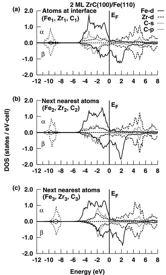
Fig. 6. Spin-polarized *site*- and *l*-projected PDOS for atoms (a) nearest, (b) second nearest, and (c) third nearest to the interface for 2 ML of ZrC on the Fe(110) substrate. These atoms are designated with subscripts 1, 2, and 3, respectively (see also Table 6).
