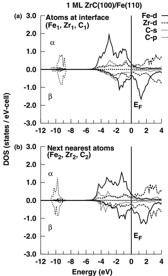
Fig. 5. Spin-polarized *site*- and *l*-projected PDOS for atoms (a) nearest, and (b) next nearest to the interface for 1 ML of ZrC on the bcc Fe(110) substrate. These atoms are designated with subscripts 1 and 2, respectively (see also Table 6). The  $\alpha$  and  $\beta$  correspond to up and down spin PDOS, where the negative PDOS values simply refer to the PDOS of the down spin electrons. The same convention is used in Fig. 6.
