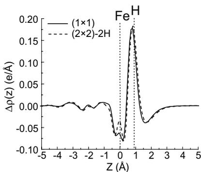
Fig. 4. Valence charge density difference integrated for planes parallel to the surface, as a function of the distance from the topmost substrate layer ( $z = 0$ ) for H in the TF site of Fe(1 1 0).
