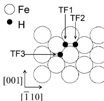
Fig. 7. Three-fold sites on Fe(110) considered for surface diffusion of H.
