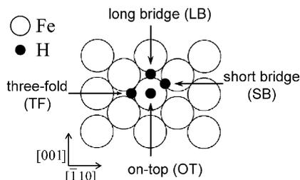
Fig. 1. High symmetry adsorption sites on Fe(110).
