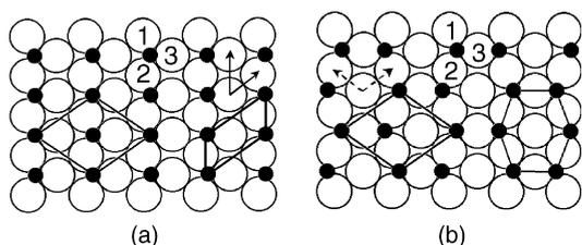
Fig. 2.  $\theta_{\text{H}} = 0.5$  ML adsorption structures of H (solid circles) on Fe(110) (open circles): (a) the  $(2\times 1)$  phase and (b) the  $(2\times 2)$ -2H phase. The hexagonal (graphitic) unit cell of the  $(2\times 2)$ -2H phase is shown in (b).
