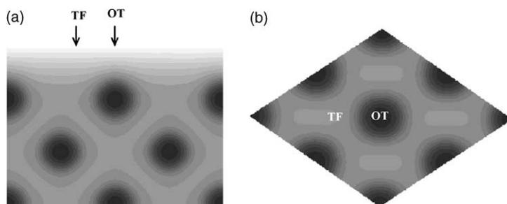
Fig. 6. Valence charge density of pure Fe(110): (a) side view from [001]; (b) top view at the surface Fe layer. Charge-density isoplanes drawn in the range of 0.01 (white) to 8.5 (black)  $e/\text{\AA}^3$  on a logarithmic scale. Fe nuclei are at the centers of the darkest regions.
