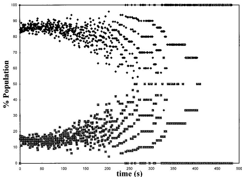
FIG. 4. The population of hydrogen atoms in the monohydride (black diamonds) and dihydride (gray squares) states versus time for a simulation at 800 K of 100 atoms with periodic boundary conditions and a defect concentration of 10% *without* the random mixing step.
