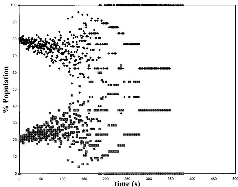
FIG. 3. The population of hydrogen atoms in the monohydride (black diamonds) and dihydride (gray squares) states versus time for a simulation at 800 K of 100 atoms with periodic boundary conditions and a defect concentration of 10% *with* the random mixing step.
