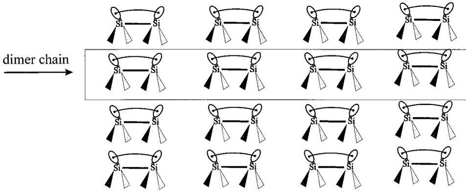
FIG. 1. The dimer chain used in the simulations is composed of dimers running perpendicular to the dimer rows on Si(100)-2 $\times$ 1.
