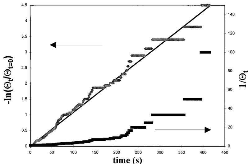
FIG. 2. Hydrogen coverage versus time for a kinetic Monte Carlo (KMC) simulation at 800 K of 200 atoms with periodic boundary conditions and a defect concentration of 10%. The data is plotted according to first-order (left axis) or second-order (right axis) kinetics. The solid line is a linear-least-squares line fit to the first-order kinetic plot. This plot is representative of the first-order kinetics we observe in all our simulations.
